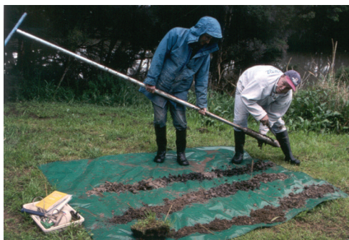
Sample collection using a hand auger 25
