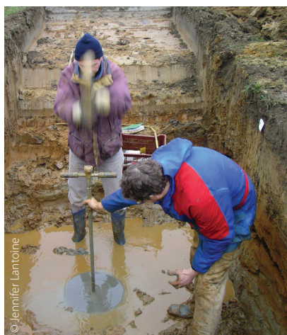
A gouge auger in action 26
