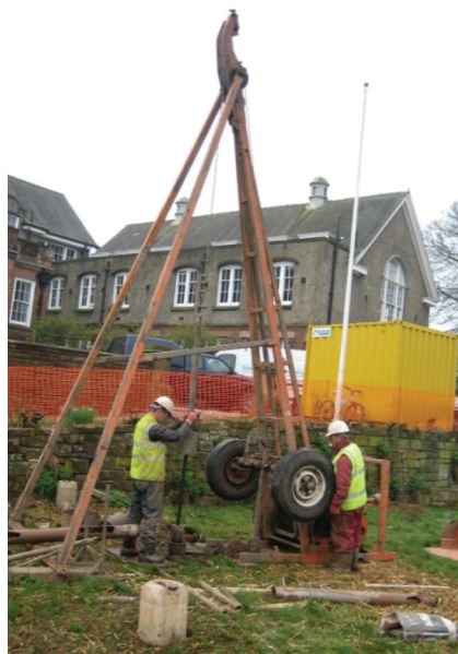
Sample collection using a cable percussion rig 28
