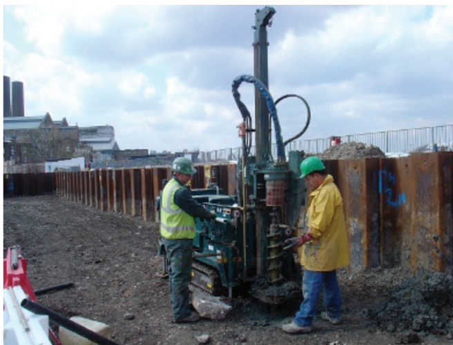
Sample collection using a rotary rig 29
